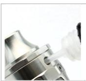
When filling the tank hold it at a slight angle so that the air can escape from the inside.
