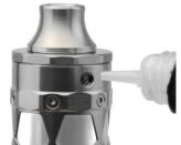
Insert the tip of the liquid bottle as straight as possible into the filling opening.
