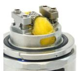
You can also roll up the cotton slightly to make sure that the channels are completely covered.
