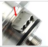
The top of the Air Disk has a small dent.
