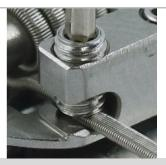
The two ends of the coil should be positioned directly below the loosened screws.
