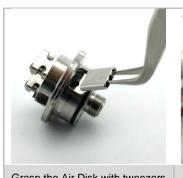
Grasp the Air Disk with tweezers for inserting/removing it.
