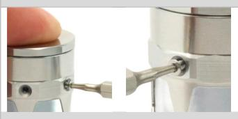
Now the other countersunk screws [R] are screwed in one after the other. (Tip: screw in "crosswise"). The top cap [S] should be pressed slightly into the tank during this process.
