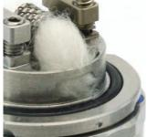
Please make sure that the cotton completely covers the channel, otherwise liquid can get into the chamber during filling.
