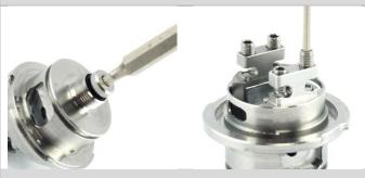
The positive pole screw [G] is now inserted through the base [C]. The positive pole screw [G] is used to fix the positive pole [E]. The four hexagon socket screws [J] can now be screwed into the coil fixings.
