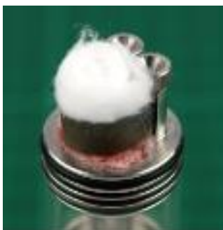
Carefully push the plug from above into the mesh arch. The mesh must not be moved or damaged.
