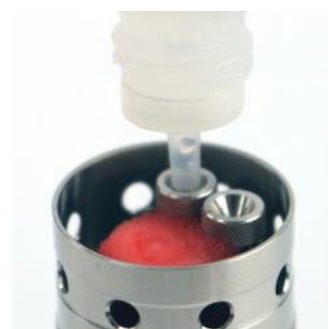
The liquid is pressed into the tank with light pressure through the bolt. The air from the tank can escape through the opening in the second bolt.
