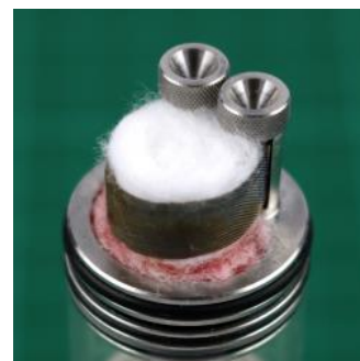
Stuff the cotton into the mesh arch. The mesh must always be in contact with the cotton.
