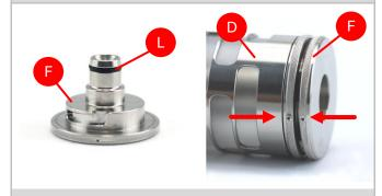
Attach the O-ring [L] to the top cap [F]. Then place the top cap [F] onto the chimney [E]. Please make sure the two alignment markings are properly positioned.
