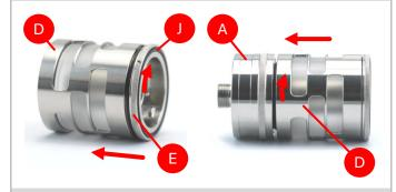
Place the O-ring [J] on top of the chimney [E]. Then screw the chimney [E] to the tank sleeve [D] and attach the assembly to the base [A].
