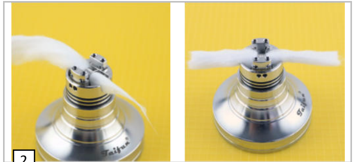
2 Pull the cotton through the coil, until both sides have the same length.
