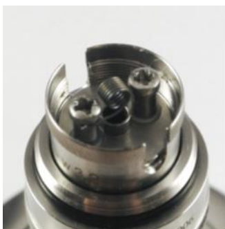
Pic. 7: It is important to make sure that the ends of the wires are not touching the chamber sleeve.
