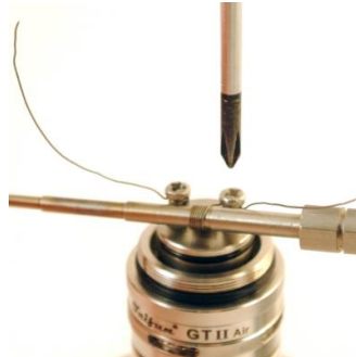
Pic 3: With a winding aid the first coil is mounted on the side and the screws tightened slightly.
