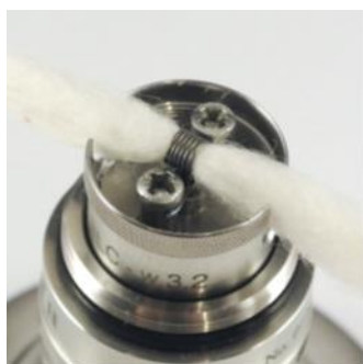
Pic. 10: You may reduce the cotton so that it fits tightly, but can still move in the winding.
