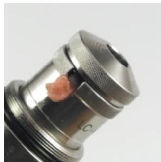
Pic. 20: The chamber cap is screwed on. Please make sure that the cotton is not cut off.
