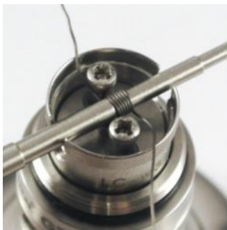
Pic. 3: Attach the wire as centrally as possible between the two poles. The wire ends should be at the bottom.
