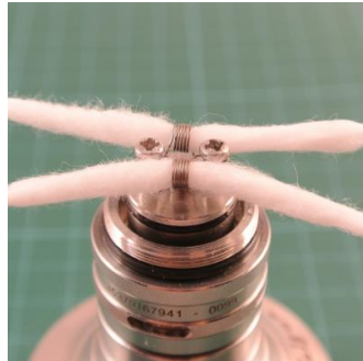
Pic 2: The cotton will be pulled through both coils.
