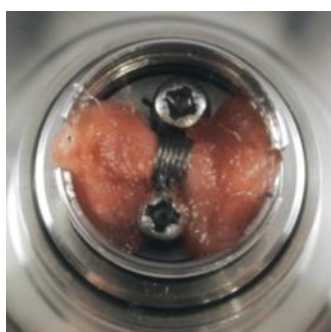
Pic. 14: The cotton wool now fills the evaporator chamber well and evenly.
