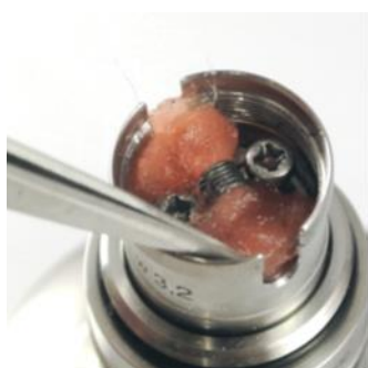
Pic. 13: Now adjust the cotton so that liquid can be well received.
