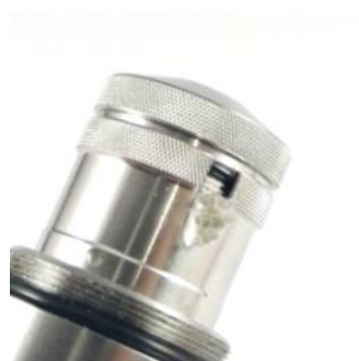
Pic. 32: The fibers should reach approximately 0.5-1 mm out of the sleeve.
