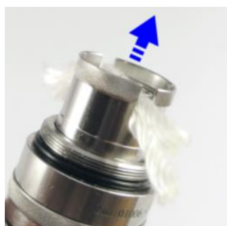
Pic. 30: The chamber sleeve is then pulled gently until it locks into place.
