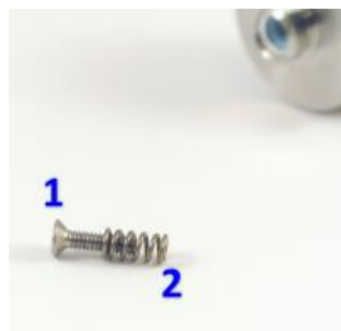
Pic 2: Therefore the countersunk screw (1) is screwed into the spring (2) first.
