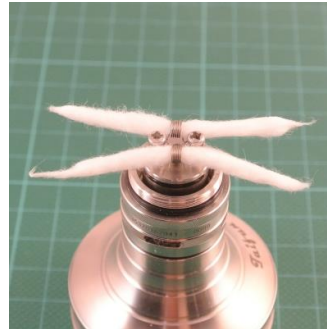
Pic 3: You may reduce the cotton somewhat by compressing the ends with the fingers slightly.
