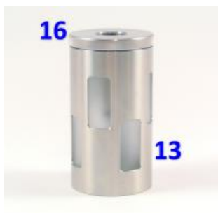
Pic 22: The glass insert (14) is fixed now inside the tank cover (13) and sealed by the o-rings (15,18).
