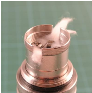
Pic 9: The cotton is cut off outside, flush with the chamber sleeve.
