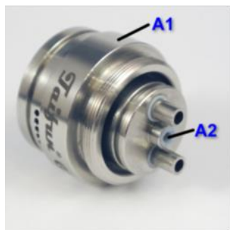
Pic. 1: The PTFE seal (A2) is inserted into the base (A1) , to reduce the air flow. This step is optional
