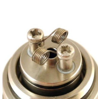
Pic 7: The distance between the two coils to the air hole should be the same.
