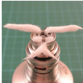
Pic 6: The ends of the cotton are placed crosswise and guided through the openings of the chamber sleeve.
