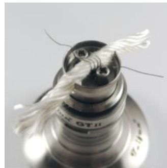
Pic. 28: After tightening the wires, the winding tool can be removed, and the winding can be corrected again, if necessary.
