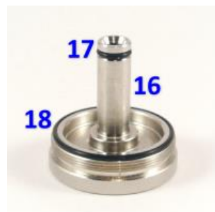
Pic 20: It is important to make sure that the o-ring (18) is not pulled over the threads of the topcap (16).
