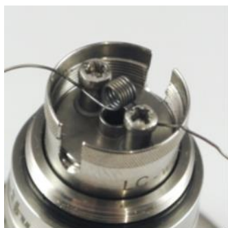
Pic. 5: Align the winding with the winding tool. Then remove the winding tool.
