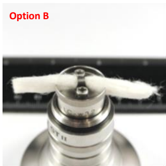
Pic. 17: The cotton is passed through the openings of the evaporator chamber to the outside.
