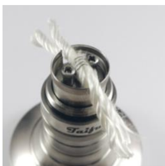
Pic. 29: The wire ends are cut flush as possible.
