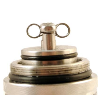
Pic 8: The upper edge of the coils should be at the height of the screw heads.
