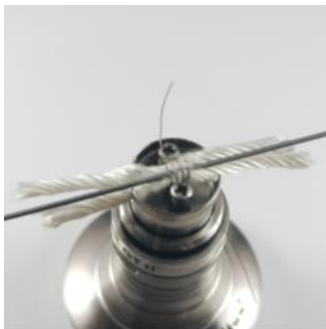
Pic. 27: Using a winding tool (e.g. a paper clip), the winding is aligned.
