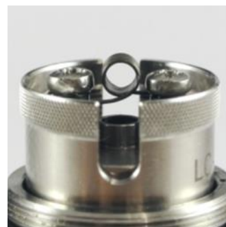
Pic. 8: The coil should now be exactly in the middle and floating around 1-1.5mm over the air hole.
