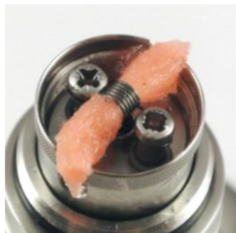
Pic. 18: The cotton is wetted with liquid, and shortened laterally so that approx. 0.5-1 mm gets outside the evaporation chamber.
