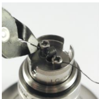
Pic. 6: The wires now shorten both sides with a pliers or other suitable tool.
