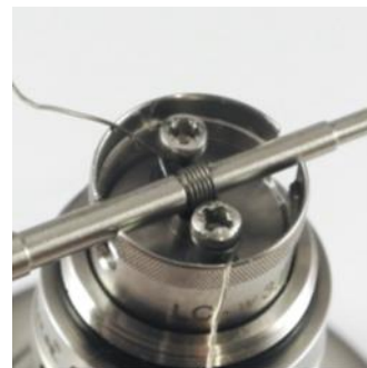
Pic. 4: The wire is placed under the screws. These are then tightened carefully.
