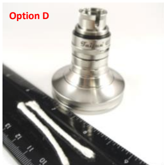
Pic. 25: A winding with silicate fiber (e.g. 3mm) is also possible.
