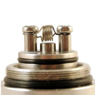
Pic 9: Also the distance to the screws should be identical for both coils.
