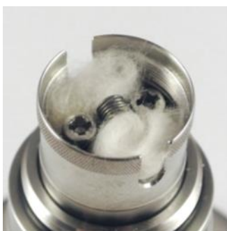
Pic. 11: Spread the cotton inside the evaporator chamber.
