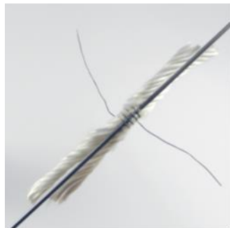
Pic. 26: In this example, the fiber is taken twice and wrapped with 32 gauge NiCr wire.
