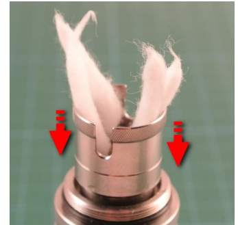
Pic 4: The cotton is folded up and the chamber sleeve is pulled over it.
