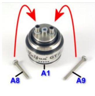
Pic. 7: The two screws for the negative pole (A8) and the positive pole (A9) can be inserted in the appropriate tubes in the base (A1) .
