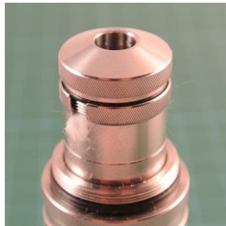
Pic 10: Now you can screw on the chamber cap.
