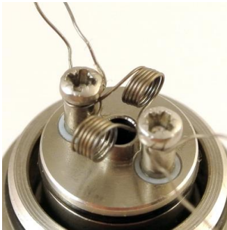
Pic 5: Once the screws have been tightened, the winding aid can be removed.
