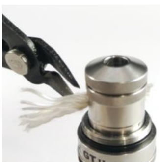
Pic. 31: Overhanging fibers are cut off on both sides.
