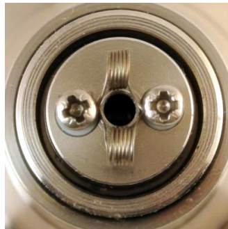
Pic 10: The windings must not touch the chamber sleeve.
