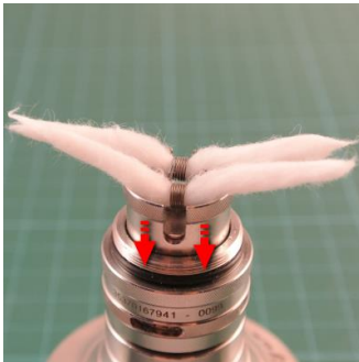
Pic 5: Push the chamber sleeve into the base now.
