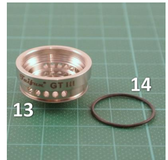
Pic 24: The O-ring [14] is now installed on the base [13].
