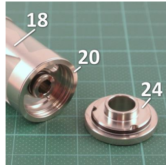
Pic 46: The top cap [24] can now be screwed onto the tank ring [20].
