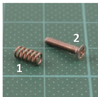
Pic 9: The countersunk screw [2] is now pushed into the spring [1].
