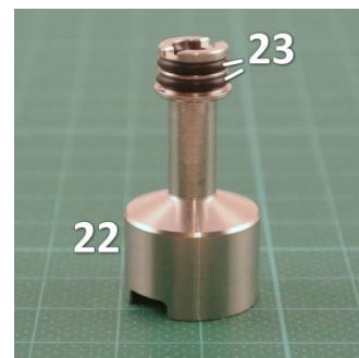
Pic 32: The O-rings [23] should now be seated, as on this pic..
