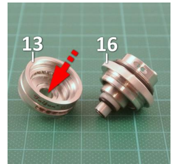
Pic 28: The deck [16] can now be inserted into the base [13].
