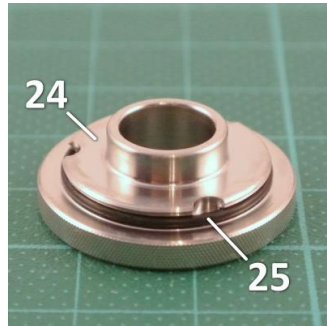
Pic 46: In the top cap [24] there is a corresponding recess for the O-ring [25].
