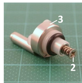
Pic 11: Put the screw [2] into the positive-pole base [3] at the bottom.
