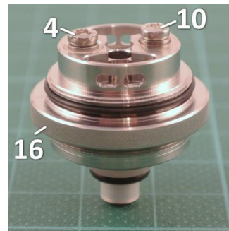
Pic 23: The positive pole [4] is now at the same level as the negative pole [10].
