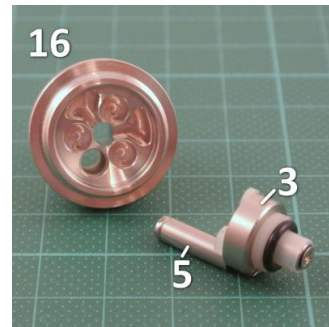
Pic 22: The positive pole base [3] is inserted from below into the deck [16]. The spacers are then positioned exactly in the recesses.
