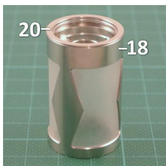
Pic 41: The tank ring [20] should now sit correctly on the tank cover [18].
