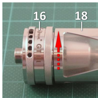
Pic 53: Both parts are now screwed together.
