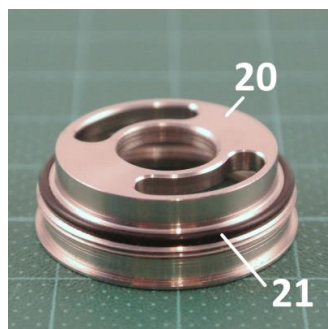
Pic 34: For this purpose there is a fine edge on the tank ring [20] in which the O-ring [21] should be seated.
