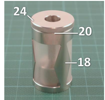
Pic 47: Top cap [24], tank ring [20] and tank cover [18] should be flush with each other.
