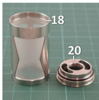
Pic 39: The tank ring [20] is now placed on the tank cover [18] ...
