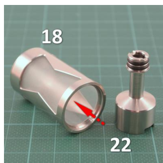
Pic 42: Now insert the chimney [22] into the tank ring [20] through the tank cover [18].
