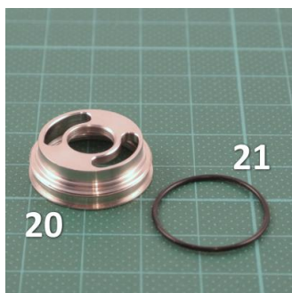
Pic 33: The O-ring [21] is now attached to the tank ring [20].
