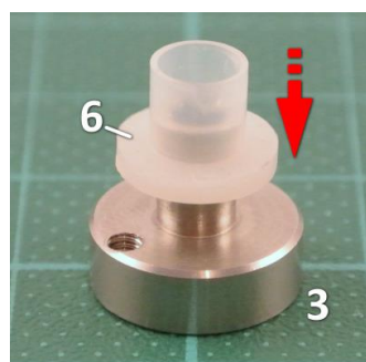
Pic 1: The isolator [6] is pushed over the positive pole base plate [3].
