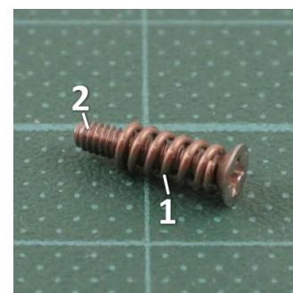
Pic 10: Push the spring [1] as far as possible onto the screw [2].
