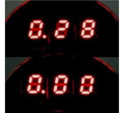
Now mount the atomizer with the short-circuit. If a valid ( $<1 \Omega$ ) resistance is detected, it will be displayed. If the measured value is stable over several seconds, the device will now be calibrated and displays ("0.00").
