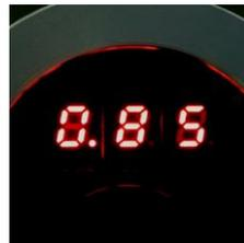
Turn the device around, and you will see the exact resistance of the coil.
