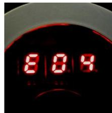
"E04" the measuring device hasn't recognize any stable value during calibration. Please clean all contacts (atomizer and device) and try again.
