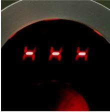
"---" the device waits for you to screw on a atomizer.
