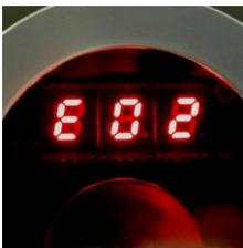
"E02" the measuring device has detected an invalid resistance. The resistance is higher than 3  $\Omega$ .
