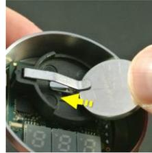
Now, press the new lithium cell CR2032, with the positive pole visible for you, between the wire bracket and the battery holder until the battery slips into the battery holder. Please don't use any tools.
