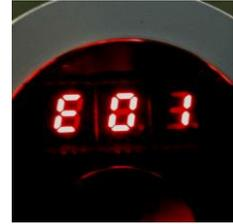
"E01" the measuring device has detected a resistance which is lower than possible by the calibration  $<0 \Omega$ . Please recalibrate!
