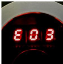
"E03" the measuring device has not detected a calibration resistance or it is outside the range of 0-1  $\Omega$ .
