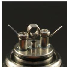
Now remove the short-circuit of your atomizer and replace it with the proper coil.
